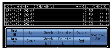
Touch switches for the alarm display (system)
